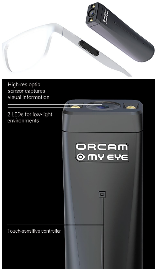
Fig. 1 OrCam device, consisting in a miniature camera, Bluetooth and Wi-Fi connectivity, includes the button for turning on and off the device and a slide bar, recognizable by touch, for managing volume, functions and settings
