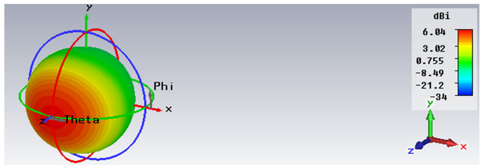
Fig. 14 Directivity for double substrate antenna with DGS
