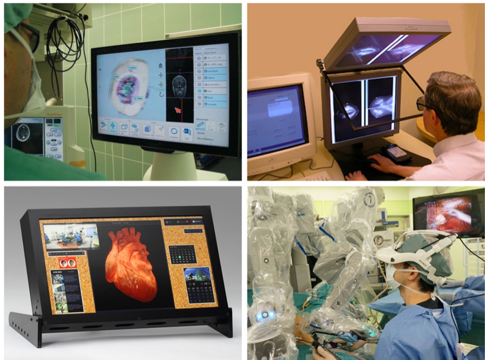
Fig. 1 3D displays in medical applications: The DexVue screen (top left) using active shutter 3D technology, Planar StereoMirror SD2250 (top right) passive stereoscopic display system, Tianma NLT autostereoscopic display (bottom left), and Sony HMM-3000MT (bottom right) head mounted display
