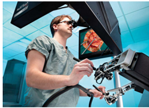
Fig. 8 Neurosurgery resident testing a NeuroTouch prototype [46]. The workstation implements a stereoscope as an immersion device to help the user locate himself in the virtual world. The system uses two Freedom 6S ® haptic devices. Picture comes from the National Research Council Canada
