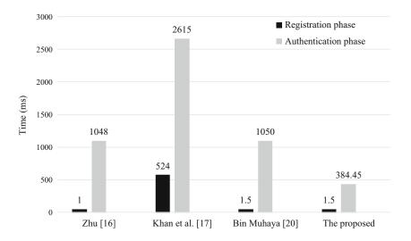
The proposed scheme in the registration phase requires three hash function operations and one exclusive-or operation; therefore, the computational cost of the registration phase is  $3h_t + 1x_t$ . During the authentication phase of the proposed scheme, six elliptic curve point multiplication operations, twelve hash function operations, and five exclusive-or operations are required. Therefore, the computational cost of the authentication phase of the proposed scheme is  $6pm_t + 12h_t + 5x_t$ .
