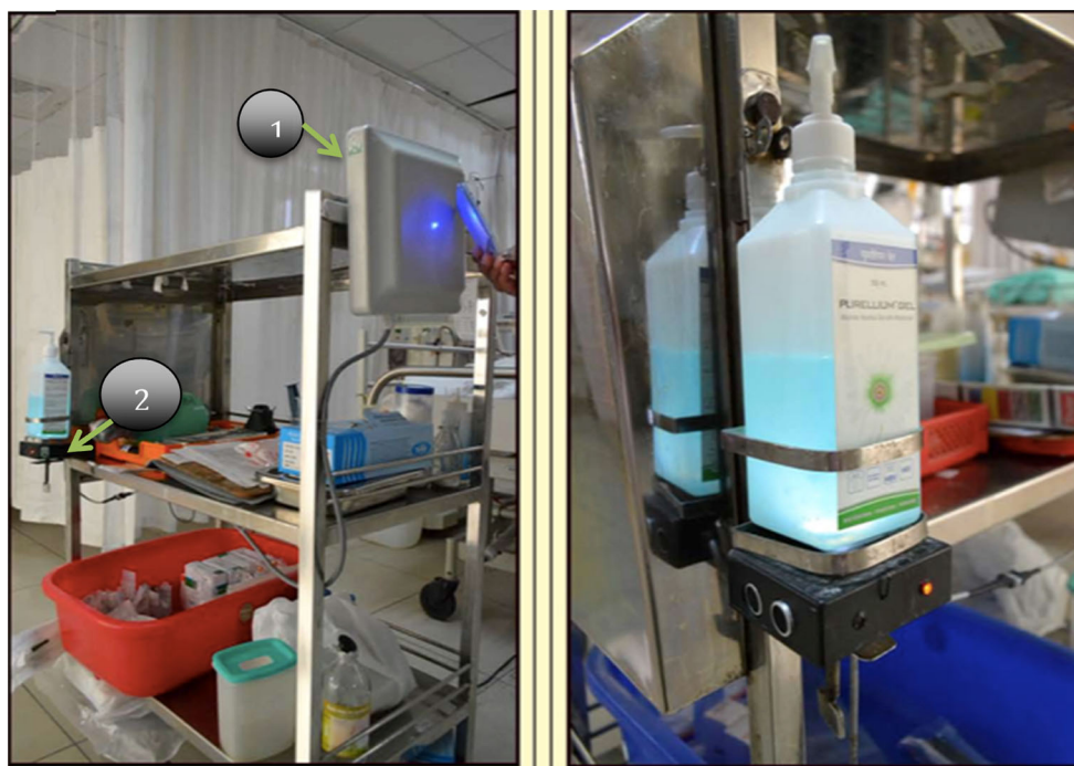
Fig. 1 a Patient trolley with the RFID reader (1) and sanitizer module (2). b Close-up of the hand sanitizer module with the glowing LED
