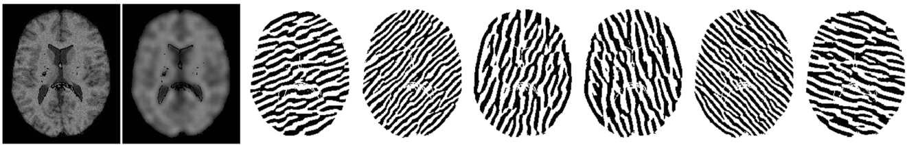
Fig. 1 A low-frequency subband and six high-frequency subbands which are oriented at 75°, 45°, 15°, -15°, -45°, -75° by the 3 level DT-CWT of the simulated brain MR image slice (z=86) shown on the left
