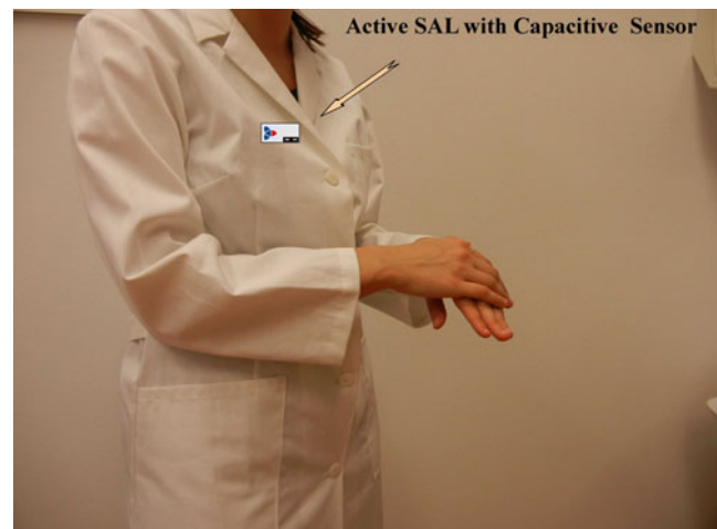
Fig. 3 Differential-dynamic disinfection mechanism, (DDM), with staff-personal sensor-tag, where the individual tagging of the ethanol level, temperature, and time stamp is executed [15, 19]. The reader, based on the IDS-902DRM interrogator chip, then provides traceability and tracks the staff's movement
