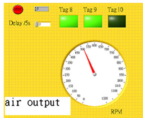
Fig. 2 Layout of the HEPA air control system. Tag8 and Tag9 are shown in green color, meaning that medical staffs with Tag8 and Tag9 entered into the room. The panel indicates the airflow volume which was regulated by the control system according to the numbers of people and the patents in the room. The air output are classify into high, median, and low. During the midnight or weekend, when the ORs are empty, the air output turn into low. During prepare time, or only one medical staff stay in ORs, the air output can automatically turn into median. When more than two patient/medical staffs are going inside ORs, the air output turn into high volume
