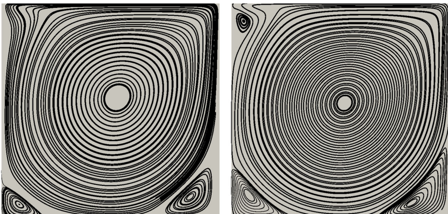
Fig. 1 Streamlines: Re = 1000 (left) and Re = 3200 (right)
