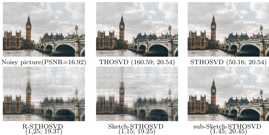
Fig. 8 Results comparison on LONDON picture with a size of 4775 \times 7155 \times 3 and white Gaussian noise in terms of CPU time and PSNR. The target rank is (50,50,3)
