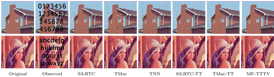
Fig. 5 The results of images House and Lena with structural missing entries described by the black letters by SiLRTC, TMac, TNN, SiLRTC-TT, TMac-TT, and MF-TTTV, respectively
