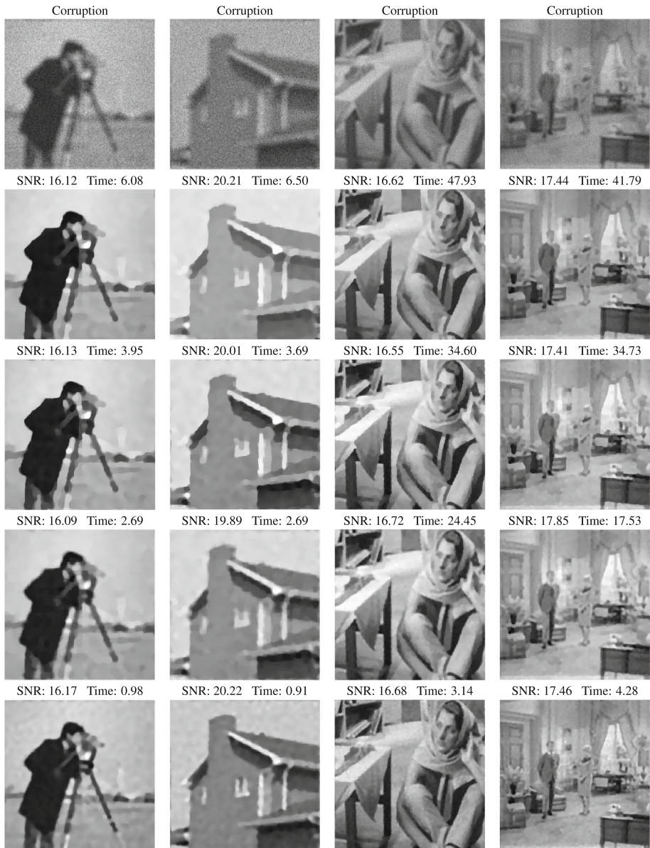
Fig. 2 Recovered images (with SNR(dB) and CPU time(s)) of different algorithms on the Cameraman, House, Barbara and Livingroom images corrupted by Average blur and Poisson noise with peak intensity M = 80 and c = 10 . First row: Noisy and blurry images. Second row: Images recovered by PIDAL. Third row: Images recovered by PIDSplit+. Fourth row: Images recovered by PD. Fifth row: Images recovered by Algorithm 1
