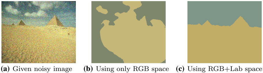
Fig. 1 Segmentation results for a noisy image (a) without the dimension lifting in Stage 2 (b) and with Stage 2 (c)
