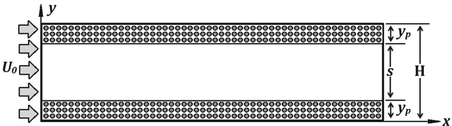
Fig. 7 Schematic of partially porous conduits with homogenous porous layer attached the walls
