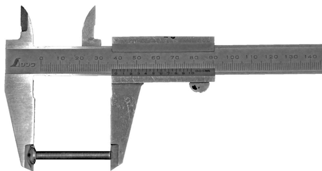
Fig. 2 Modified caliper for measuring the functional vertebral length. This was made by following the method proposed by Taylor and Wedel (2013b). The bolt was glued onto the left jaw of the caliper so that it lay perpendicular to the other jaw
