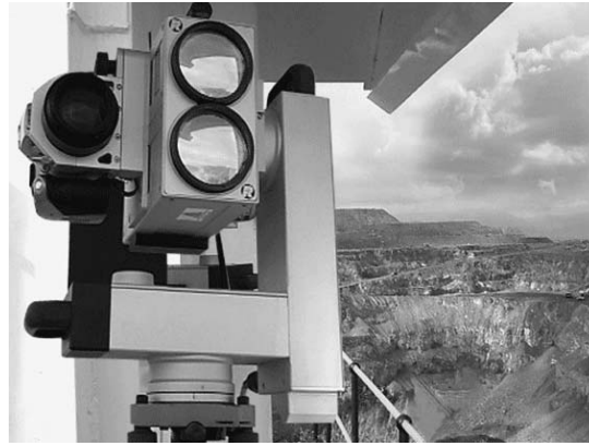
Fig. 2. Riegel LPM-2K SiteMonitor by 3-D Laser Mapping Ltd U.K.
