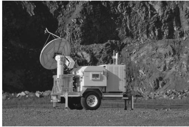
Fig. 4. Movement and Surveying Radar, MSR 300 [24]
