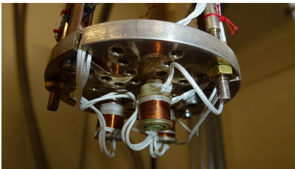
Fig. 1 The three specimens of quartz tuning forks placed inside their copper holders with additional superconducting coils for the modulation of magnetic field. All of them are mounted on the experimental plate of cold finger of the cryogen-free dilution refrigerator Triton 200 (Color figure online)
