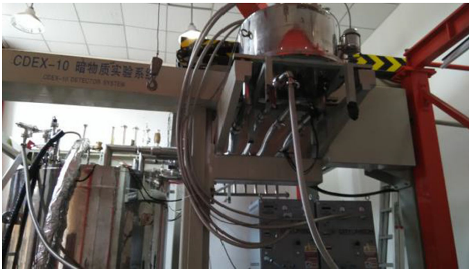
Fig. 8 The cryogenic system of CDEX-10 (Color figure online)
