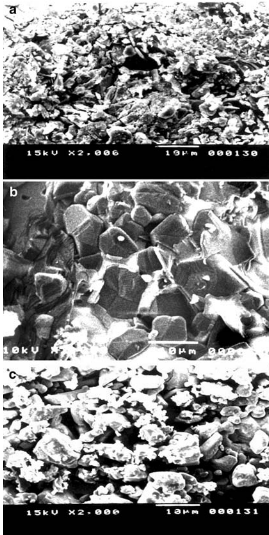
Fig. 6. (a) Surface morphology of the powder compacts of the \text{Bi}_{1.82}\text{Pb}_{0.36}\text{Sr}_2\text{Ca}_2\text{Cu}_3\text{O}_y . Surface morphology of the powder compacts of the \text{Bi}_{1.82}\text{Pb}_{0.36}\text{Sr}_2\text{Ca}_2\text{Cd}_{0.35}\text{Cu}_3\text{O}_y . Surface morphology of the powder compacts of the \text{Bi}_{1.82}\text{Pb}_{0.36}\text{Sr}_2\text{Ca}_2\text{Cd}_{0.55}\text{Cu}_3\text{O}_y . (a–c) Surface morphology of the powder compacts of the \text{Bi}_{1.82}\text{Pb}_{0.36}\text{Sr}_2\text{Ca}_2\text{Cd}_x\text{Cu}_3\text{O}_y , (a) Cd ( x=0.0 ), (b) Cd ( x=0.35 ), (c) Cd ( x=0.55 ).
