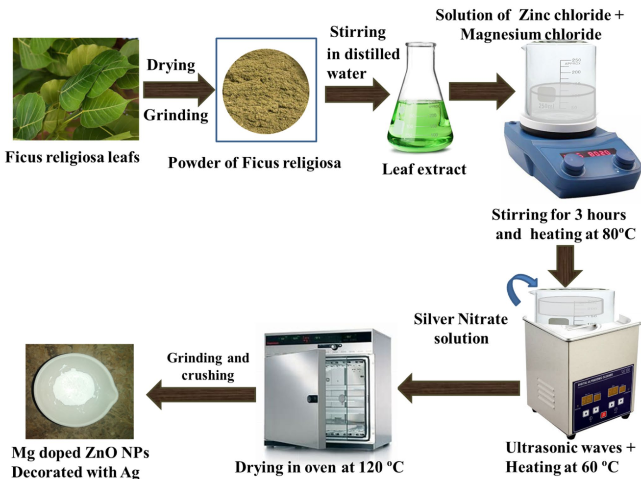
Fig. 1 Presents green's synthesis process of Mg doped ZnO decorated with Ag
