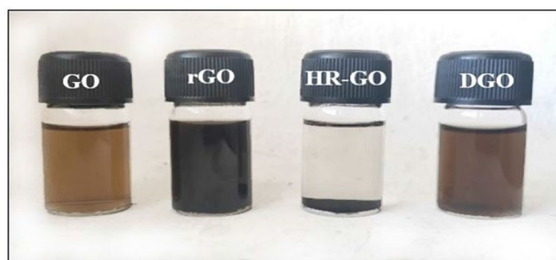
Fig. 2 Digital photograph of GO, rGO, HR-GO, and DGO. GO graphene oxide, rGO reduced graphene oxide, HR-GO hydrazine reduced graphene oxide, DGO distilled water reduced graphene oxide
