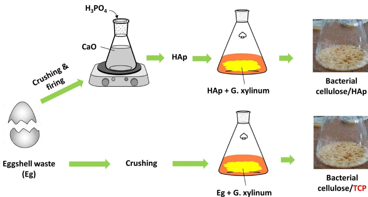
Fig. 1 Schematic representation of synthesis of different composites based on BC and eggshell or eggshell-derived HAp
