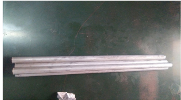
Fig. 1 Al7075 raw material for the stir casting process
