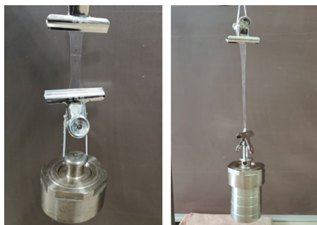
Fig. 3 a PU-600 sample with different weight suspending (from left to right are 850 g and 2225 g loadings, respectively), and this sample was heated at 50 °C for 2 h
