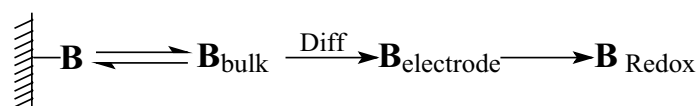
Scheme 2 Schematic presentation of the desorbing electrochemical process with the binding molecule B
