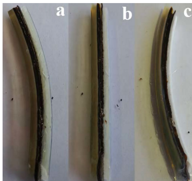
Fig. 7 Shape changing with temperature at the artificial reactor SVA-AmAg-SI ( a 25 °C; b 35 °C; c 45 °C)
