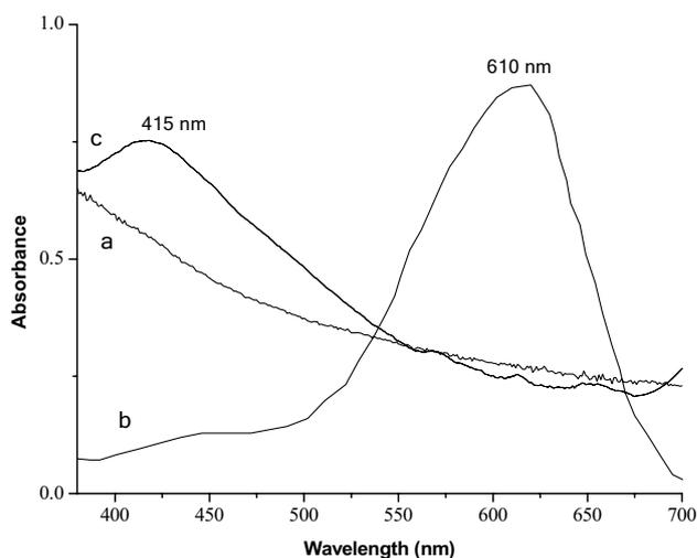
**Fig. 1** The UV–Vis absorption spectrum of the extracted solution of (a) pristine wool sample, (b) indigo-dyed wool sample, and (c) silver treated indigo-dyed wool sample
