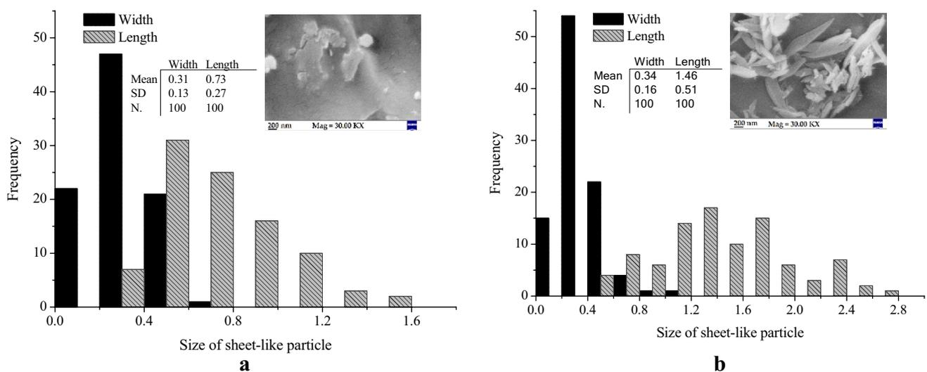
**Fig. 3** The size distribution histograms of platelet-like particles of indigo colorant for **a** silver pre-treated indigo-dyed wool sample and **b** simultaneous silver treated indigo-dyed wool sample during the dyeing process
