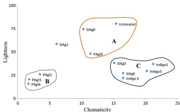
**Fig. 7** The chromaticity and lightness of un-treated and silver treated indigo-dyed wool samples. The yellow and brown samples located at zone A, while silver pre-treated indigo-dyed wool samples had the lowest chromaticity and lightness located at zone B and blue dyed samples stayed on zone C (Color figure online)
