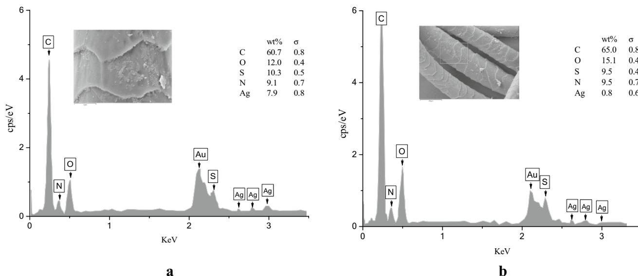
**Fig. 4** The EDS spectrum of wool fiber samples which are **a** silver pre-treated indigo-dyed wool sample and **b** simultaneous silver treated indigo-dyed wool sample during the dyeing process. The insert SEM images indicated the area selected for EDS analysis
