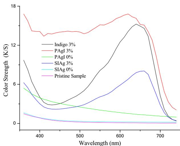
**Fig. 8** The color strength (K/S) spectra of un-treated and silver treated indigo-dyed wool samples (Color figure online)
