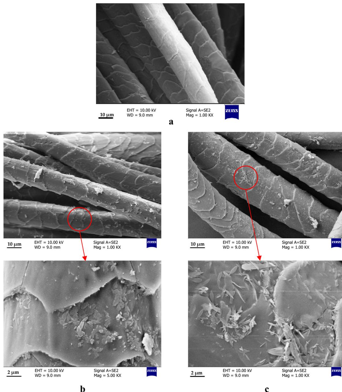
**Fig. 2** The SEM images of wool fiber surface which are **a** pristine fiber sample, **b** silver pre-treated indigo-dyed wool sample and **c** simultaneous silver treated indigo-dyed wool sample during the dyeing process
