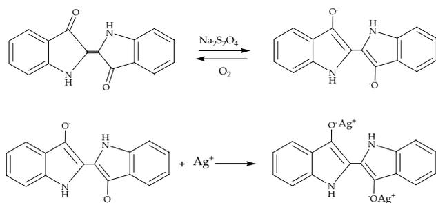
**Fig. 5** Proposed interaction mechanism of silver with water-soluble *leuco*-form of indigo molecular
