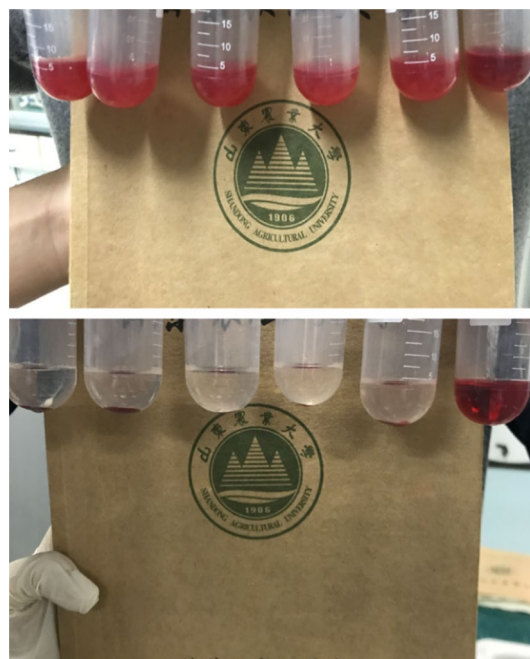
Fig. 13 Photographs of hemolysis test. The top figure shows the samples that were incubated at 37 °C, and the bottom figure shows the supernatant sample to be tested after centrifugation. The centrifuge tubes from the left to right are samples 1–6. Sample 1: the normal saline solution, samples 2–5: PNIPA/HA-2 to PNIPA/HA-5, sample 6: distilled water
