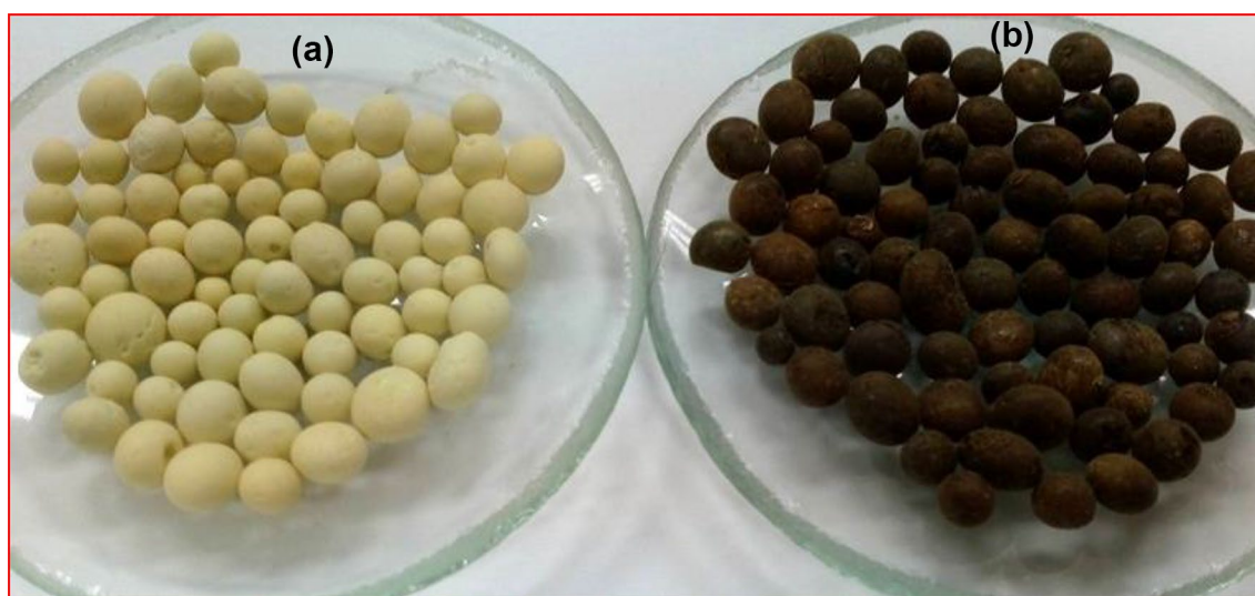
Fig. 1 Photo images of an aluminum substrate (a), and MnO 2 -coated aluminum substrate (b)
