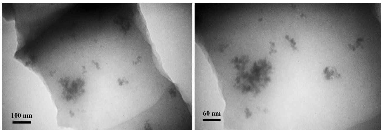
Fig. 6 TEM image of PIEN 10b nanocomposite
