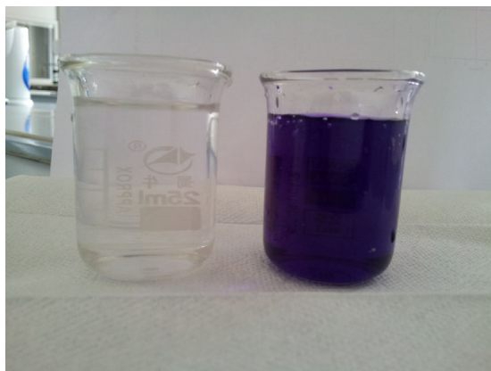
Fig. 6 a UV-visible spectra for degradation of MV in aqueous solution containing SrFe 12 O 19 /Zn 0.65 Ni 0.25 Cu 0.1 Fe 2 O 4 core-shell nanocomposite, b for subsequent five runs, c color of MV is violet but after catalysis it turned as colorless (Color figure online)
