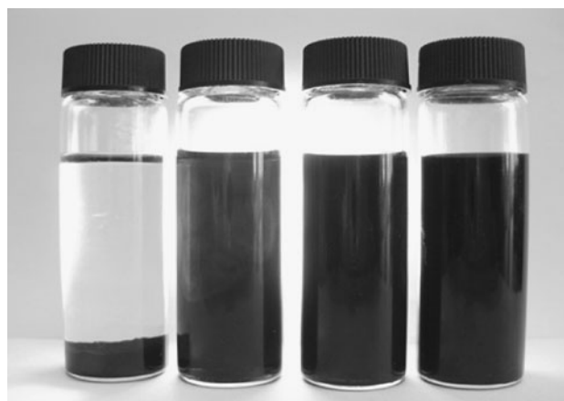
Fig. 6 Covalent multifunctional SWNT dissolution in DMF after sonication; from left to right: p-SWNT, 1a , 2a , 3a
