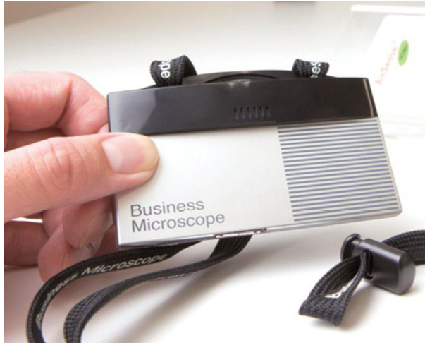
Fig. 1 The present study's sociometric badges from the Hitachi Research Lab
