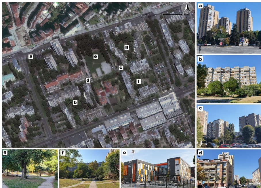
Fig. 3 Micro-unit in Liman III: population—approx. 4000, area—11.6 ha (housing—9 ha), population density—approx. 450 inh/ha (calculation based on GeoSrbija spatial data); a and b first housing towers and slabs; c dominance of ‘gray modernism’; d rooftop expansions; e music and ballet school built in place of sports fields and greenery (opened in 2021); f tucked up inner-block pedestrian paths; g inner-block greenery. Source: aerial view—GeoSrbija ( https://a3.geosrbija.rs/ ); photos—authors
