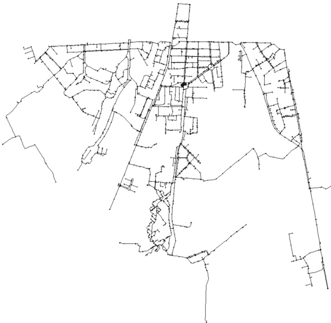
Fig. 5 EPANET model of the Pressure Management Zone (PMZ) “Abbategrasso”, in Milan, Italy
