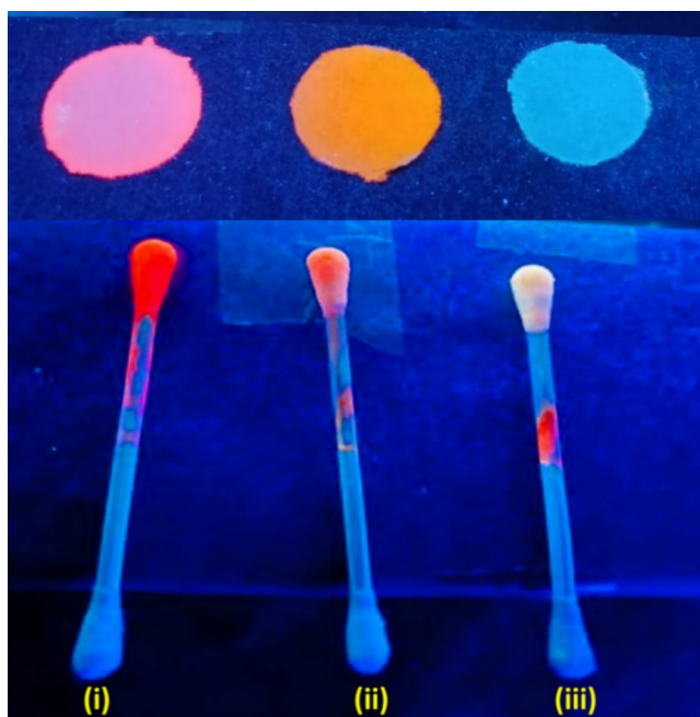
Fig. 11 Paper strips and cotton buds coated with (i) pap-AuNCs, (ii) PLP_pap-AuNCs, and (iii) PLP_pap-AuNCs in the presence of Zn^{2+} ions
