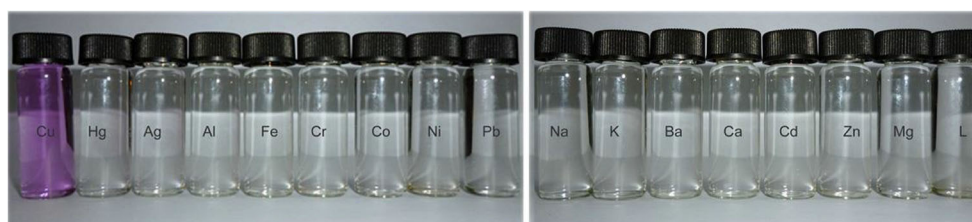
Fig. 3 Change in color of 10 \mu\text{M} 13 in \text{CH}_3\text{OH}/\text{HEPES} ( 20 \text{ mM} , \text{pH}7.2 , 1:1, \text{v/v} ) semiaqueous solution with 5-time cation from left to right: \text{Cu}^{2+} , \text{Hg}^{2+} , \text{Ag}^+ , \text{Al}^{3+} , \text{Fe}^{3+} , \text{Cr}^{3+} , \text{Co}^{2+} , \text{Ni}^{2+} , \text{Pb}^{2+} , \text{Na}^+ , \text{K}^+ , \text{Ba}^{2+} , \text{Ca}^{2+} , \text{Cd}^{2+} ,
