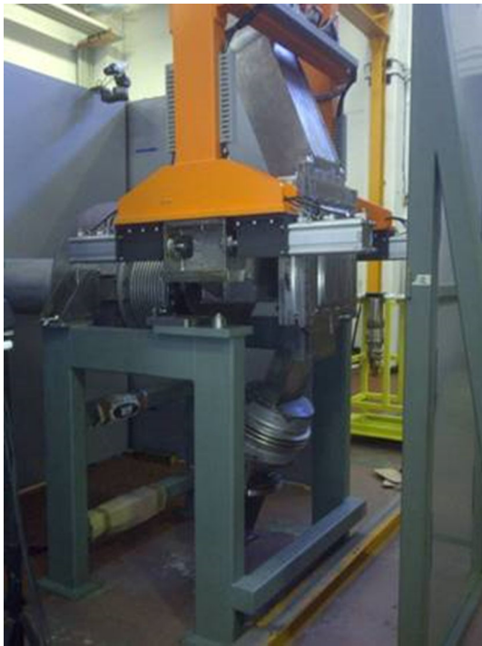
Fig. 28 RH validation tests for the replacement of the Target Assembly
