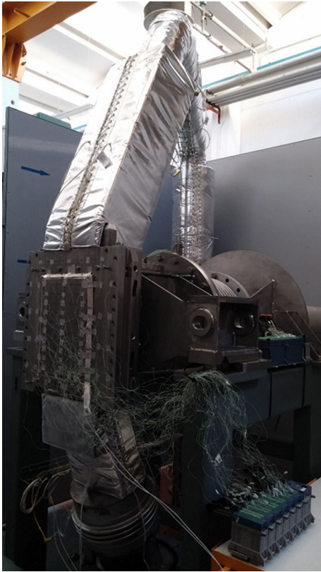
Fig. 22 Pre-heating tests on the TAA prototype at ENEA DRP laboratory
