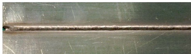
Fig. 7 The weld surface based on the new cosmetic welding parameter
