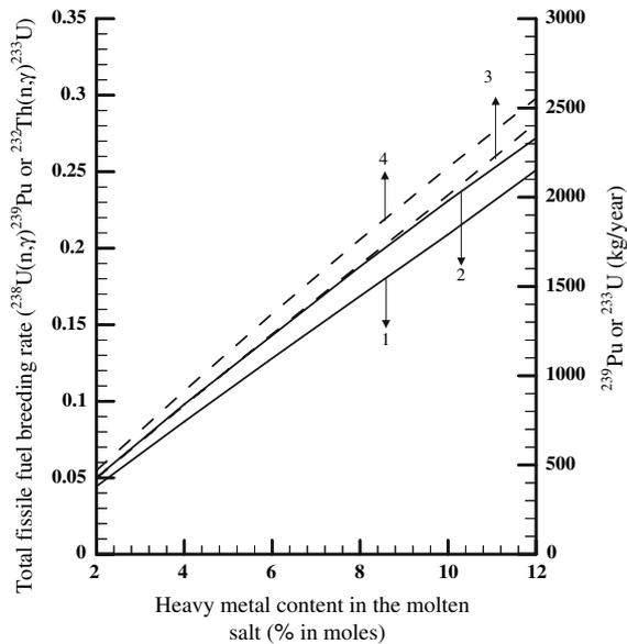
**Fig. 7** Total fissile fuel breeding rate (1)  $^{238}\text{U}(n,\gamma)^{239}\text{Pu}$ , (2)  $^{232}\text{Th}(n,\gamma)^{233}\text{U}$  and annual fissile fuel production (3)  $^{239}\text{Pu}$ , (4)  $^{233}\text{U}$  with respect to the heavy metal content
