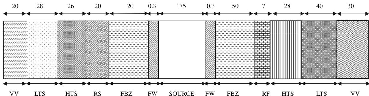
**Fig. 2** One-dimensional blanket model of the ARIES-RS fusion reactor [4]. VV, vacuum vessel; LTS, low temperature shield; HTS, high temperature shield; RS, replaceable shield; FBZ, fuel breeding zone; FW, first wall; RF, reflector (dimensions are given in cm, not in scale)
