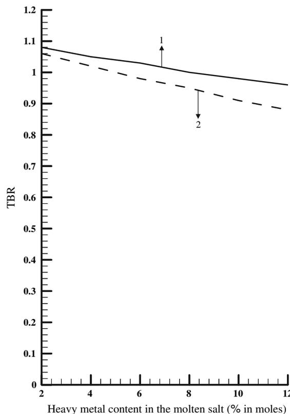
**Fig. 5** TBR variation with respect to the molten salt composition for the blanket with: (1) Flibe + UF<sub>4</sub>, (2) Flibe + ThF<sub>4</sub>
