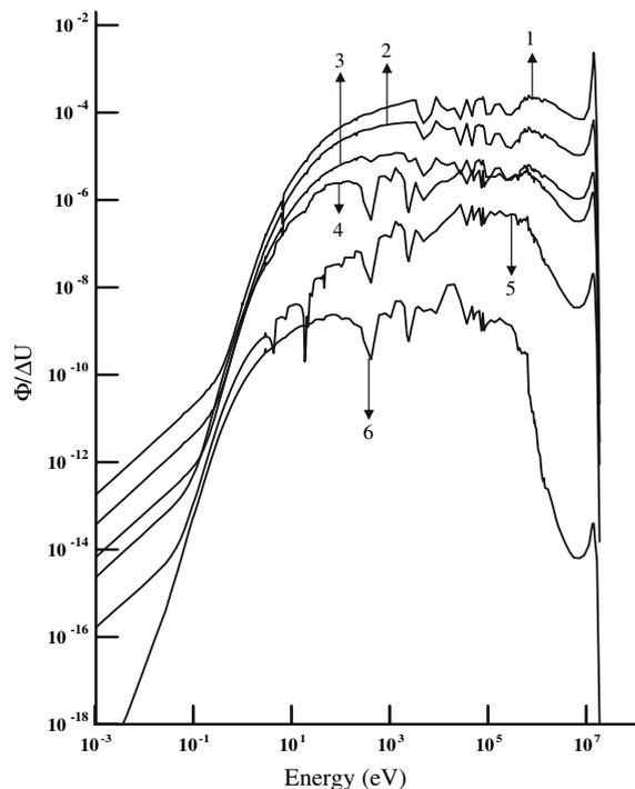
**Fig. 4** Neutron spectrum at different locations of the outer blanket with 96% Flibe + 4% UF<sub>4</sub>: (1) on the left side of the heavy molten salt zone, (2) in the middle of the heavy molten salt zone, (3) on the right side of the heavy molten salt zone, (4) on the right side of the shielding zone, (5) on the right side of the HT zone, (6) leakage spectrum
