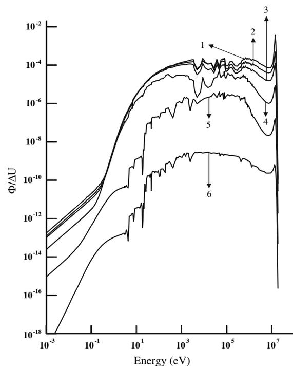
**Fig. 3** Neutron spectrum at different locations of the inner blanket using 96% Flibe + 4% UF<sub>4</sub>: (1) on the right side of the heavy molten salt zone, (2) in the middle of the heavy molten salt zone, (3) on the left side of the heavy molten salt zone, (4) on the left side of the shielding zone, (5) on the left side of the HT zone, (6) leakage spectrum
