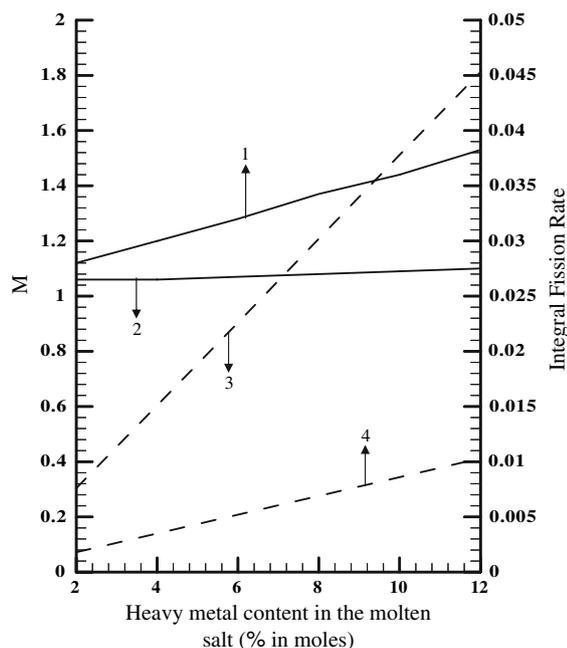
**Fig. 6** Energy multiplication versus heavy metal content with (1) Flibe + UF<sub>4</sub>, (2) Flibe + ThF<sub>4</sub> and integral fission versus heavy metal content with (3) Flibe + UF<sub>4</sub>, (4) Flibe + ThF<sub>4</sub> (per incident fusion neutron)
