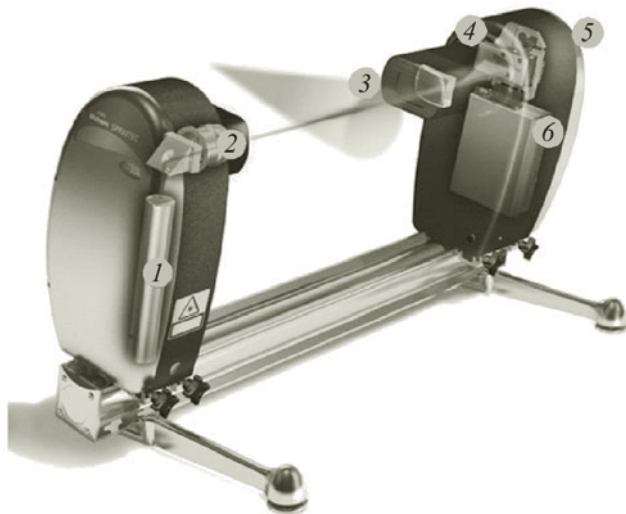
Fig. 2. Measuring Malvern Spraytec system: 1) He–Ne laser; 2) collimated optics; 3) droplet flow; 4) Fourier lens; 5) detector based on silicon diodes; 6) high-speed system for data collection.
