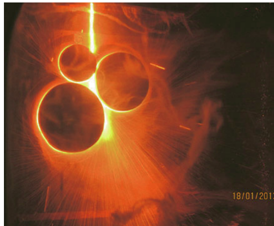
Fig. 6. Inflation of the basalt melt jet into fiber with the aid of a three-roll centrifuge.
