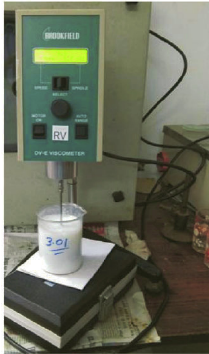
Fig. 6. RVDV-E viscometer for measurement of the TiO 2 nanofluid viscosity.
