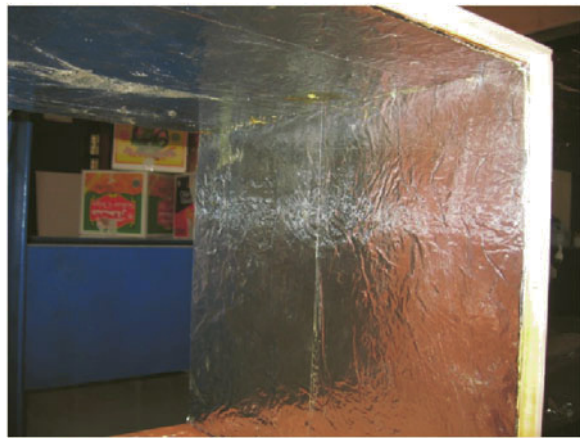
Fig. 2. Wooden box fabricated from a heat-proof material [6].
