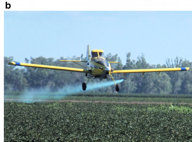
Fig. 2 a Schematic diagram of the apparatus used for aerial application of Magnet ® b Spraying in progress. Since large droplets were required, nozzles were not appropriate, and the formulation was simply pumped through a pipe under the wing, at a speed which matched the forward speed of the aircraft (AgBiTech 2016b). This produced droplets from 1 to 5 mm in diam, large enough for moths to feed on, in bands 1–2 m wide, spaced between 36 and 144 m apart, depending on anticipated pest pressure. Application by air was very quick, allowing 1000–2000 ha per hour to be treated, depending on band spacing
