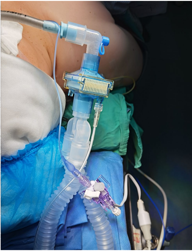
Fig. 1 A tracheal tube with a pressure transducer for continuously monitoring the cuff pressure
