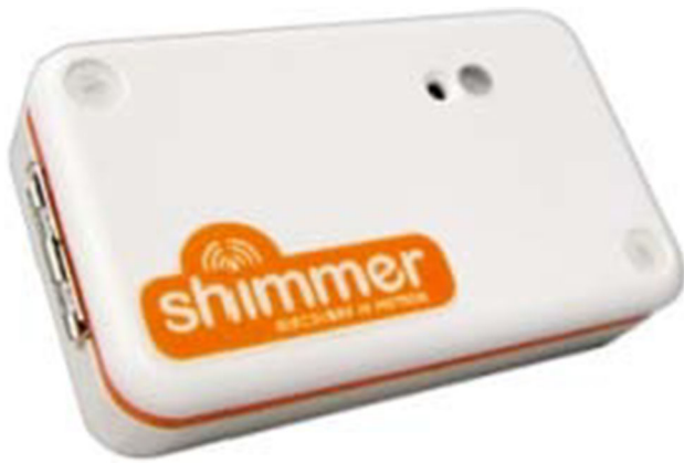
Fig. 2 Shimmer platform to facilitate wireless Bluetooth connection from sensing element to computer
