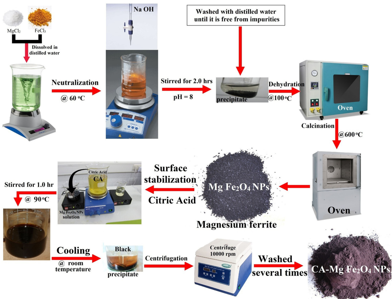
Scheme 1 The systematic representation of the synthesis and surface modification of \text{MgFe}_2\text{O}_4 NPs by citric acid (CA)
