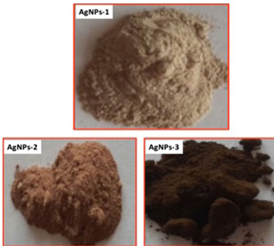
Fig. 1 Photographic images of AgNPs powders synthesized at different concentrations of silver nitrate. Where AgNPs-1 = 0.05 g AgNO 3 /0.2 g Acacia and AgNP-2 = 0.10 AgNO 3 /0.2 g Acacia and AgNPs-3 = 0.2 g AgNO 3 /0.2 g Acacia
