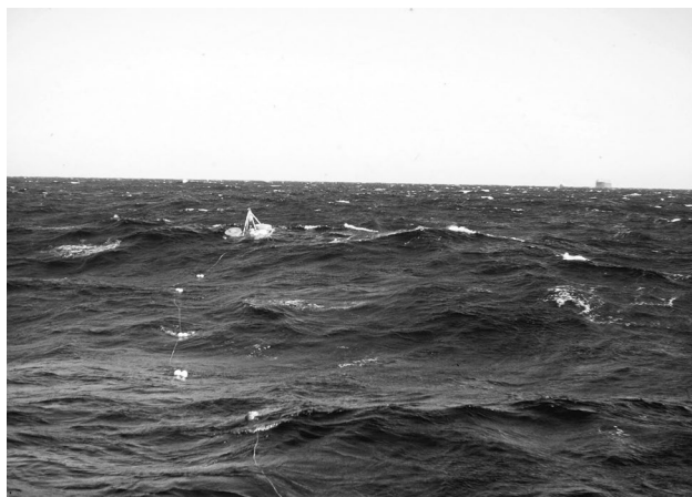
Fig. 8 Breaking waves in the North-Western Pacific Ocean during wave observations using a clover-leaf buoy (Mitsuyasu et al. 1975). Wind speed U_{10} is about 9 m/s, mean wave height is 1.5 m, and mean wave period is 6.2 s
